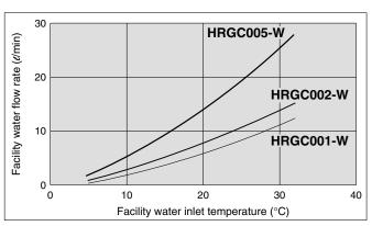
\* This is the flow rate of facility water at the rated cooling capacity and circulating fluid flow, operating at 60 Hz.
