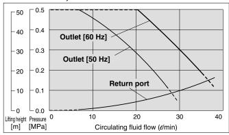
\* For all common models, temperature stability will decline in the flow rate range where circulating fluid is deduced (dotted line).
