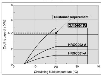
The point plotted in the graph is the requirement from your customer. Select the Thermo-cooler models exceeding this point. In this case, select the
