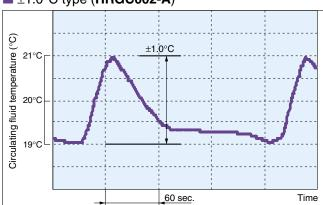
Note 3) The value shown applies to a stable load state with no outside interference. Actual values may vary depending on the operating conditions.
