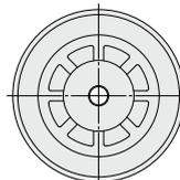
Pad diameter  $\phi 4$  to  $\phi 8$
