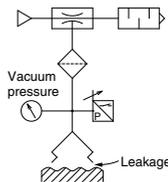
If a considerable amount of leakage occurs between the workpiece and the pad, resulting in incomplete adsorption, or to shorten the adsorption and transfer time, select an ejector nozzle with a larger diameter from the ZH, ZR, or ZL series.
