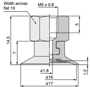
**Dimensions/With Adapter: Vacuum Inlet** **Vertical**
