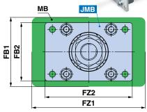
Width: Max. 20% reduction, Height: 16% reduction Dimension comparison (When mounted on the cylinder)
