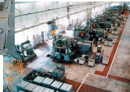
Aluminum casting machine line
