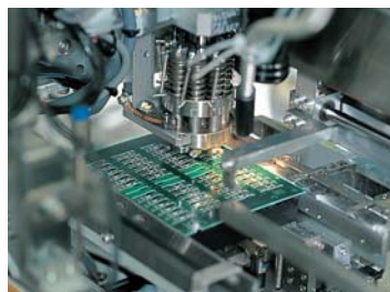
IC chip, being mounted on printed board
