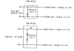
@Connection of contact protective box Connect contact protective box with the switch by using lead wire with indication "SWITCH" of the box and lead wire of the switch.
