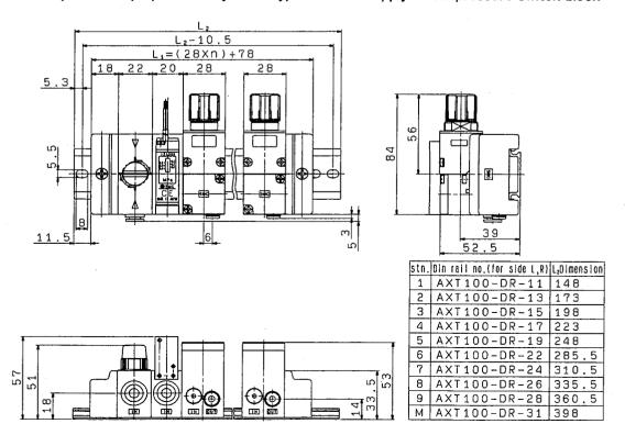
ARM11AB1 — \* 12 Handle position front spec. ∕ common supply block
