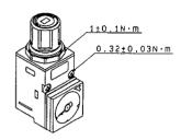
②Holding screw for reugulator assembly mounted on regulator block
