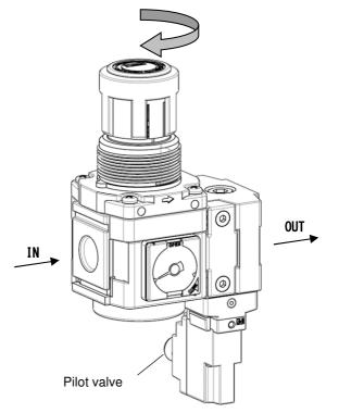
(2) Turn on the power to the pilot valve and supply pressure to the IN side of the product. Then, turning the handle clockwise in the unlocked state increases the pressure on the outlet side. Note) Always set the pressure in the upward direction (arrow direction). Otherwise, it may cause insufficient set pressure.
