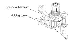
Tighten the 2 holding screws on the spacer with bracket or spacer evently. Tighten them to the recommended tightening torque. Insufficient tightening torque may result in loosening or sealing failure. Excessive tightening torque may damage the thread, etc.
