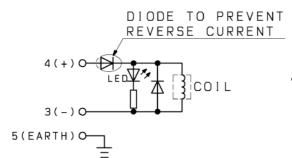
Connect correctly the lead wires to + (positive) and – (negative) indications on the connector.
