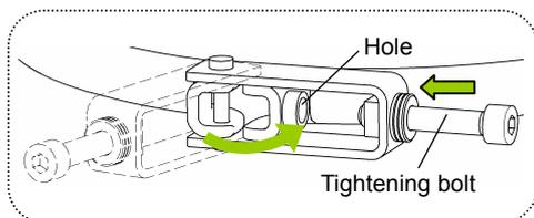
**Fig. C Position for V band bolt for tightening**
