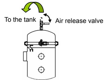
Fig. 1-2. Air release circuit
