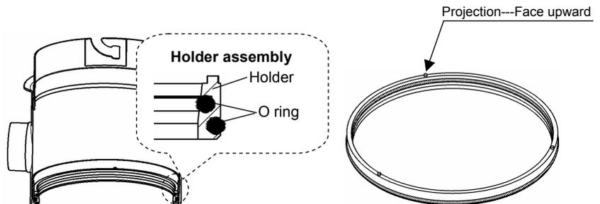
**Fig. 6-2. Holder assembly mounting direction**
