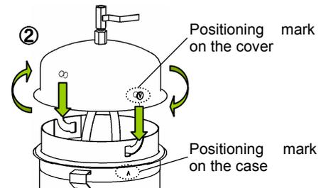
**6 [Mounting and tightening of V band]**
