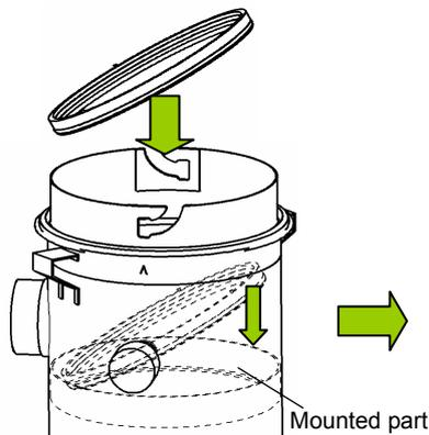
**Fig. 6-1. Holder assembly replacement**
