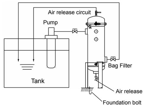
**Fig. 4-1 Example of the circulating filter circuit**
