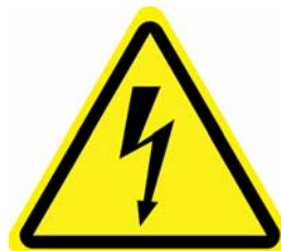
Fig. 1-2 Warning label for high voltage
