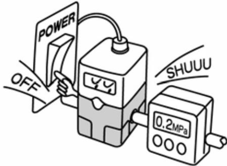
If the power supply to this product is turned off due to a power failure during normal operation, the output on the secondary side will be held and air will flow continuously.
