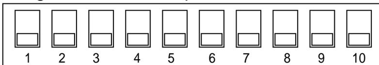
Node address: 0    Baud rate: 125kbps
