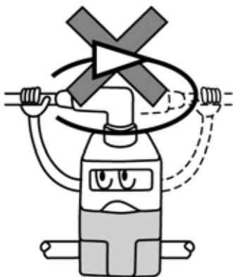
Please note that the right angled cable connector does not rotate and is limited to only one entry direction.
