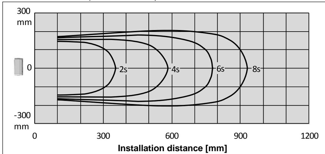
At minimum air flow (air flow scale: 1)
