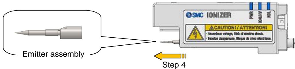
5. When mounting a new emitter assembly to the cartridge assembly, use gloves and tweezers to ensure the emitter is not contaminated. (Do not touch the emitter assembly with bare hands).
