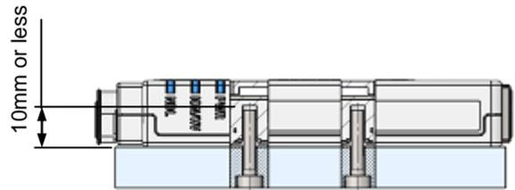
Use a screw with maximum screw-in depth of 10 mm
