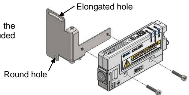
b. Fixing of the bracket
