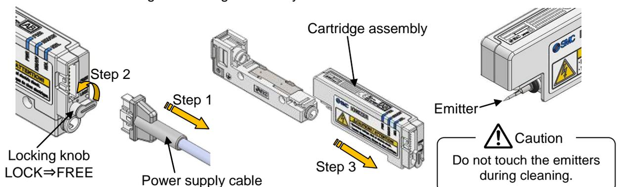
4. Clean the emitter mounted to the cartridge assembly.
