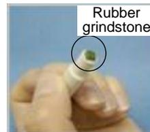
Use if dirt cannot be removed with felt.
