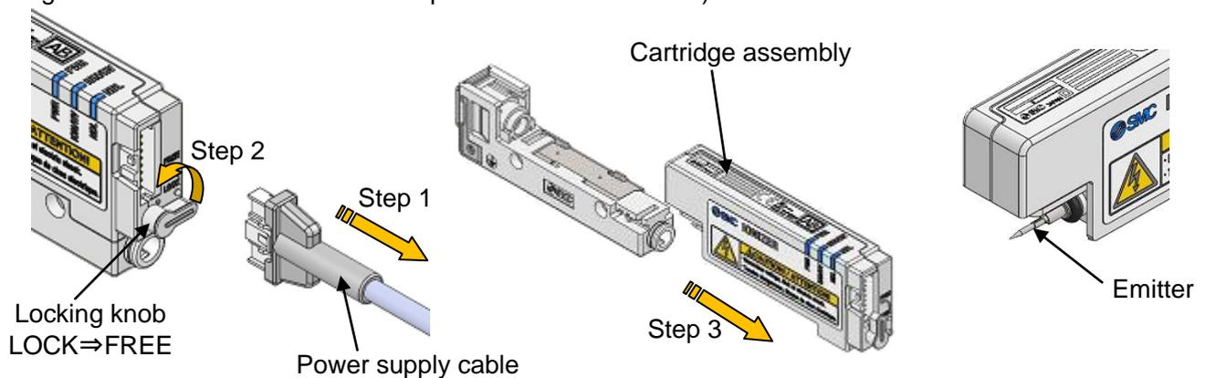
The procedure for mounting the cartridge assembly is the reverse of removal. Confirm that the Locking knob is in the FREE position.
