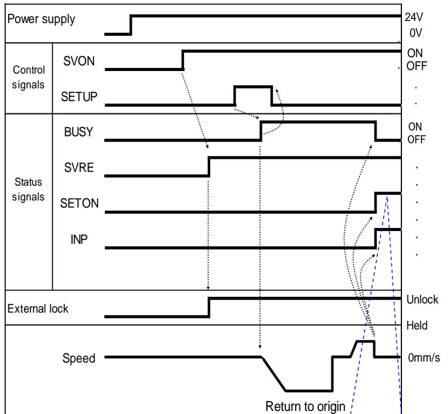
INP signal is ON when the current position is within the step data position range. Otherwise, the signal is OFF
