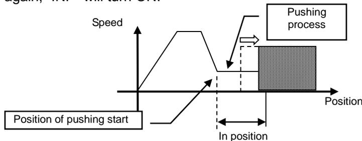
[2] Movement of the workpiece in the direction opposite to the pushing direction (The actuator is pushed back since the reaction force from the workpiece is too large.)
