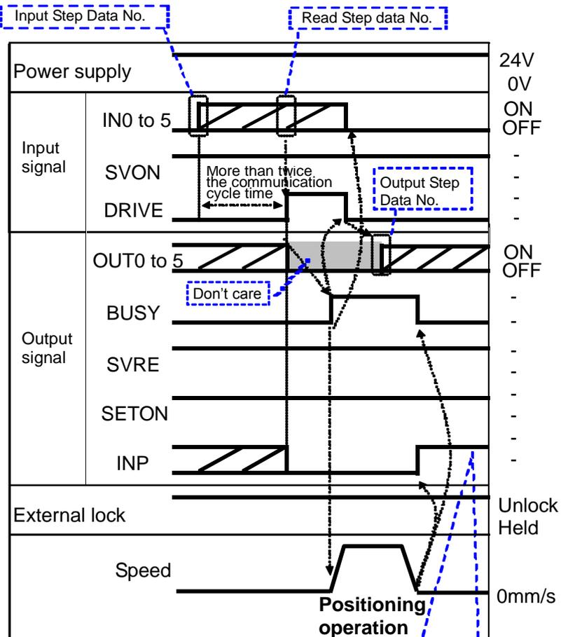
If the current position is inside of step data positioning, the INP signal is ON. Otherwise, the signal is OFF
