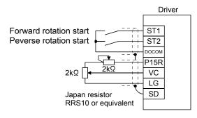
Refer to "8. Assignment of input/output signal" for assignment of signal.
