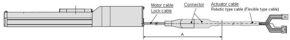
9. **Select "Robotic type cables" in case of inflecting actuator-cable repeatedly. And do not put cables into a flexible moving tube with a radius smaller than the specified value. (Min. 50mm).**
