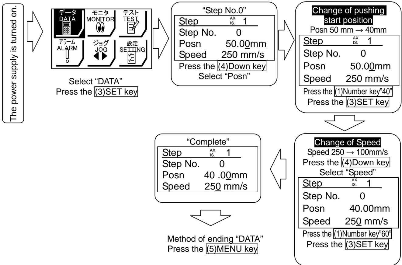
“Step No.1” / Positioning operation / At the time of shipment, Step No.1 is set to positioning operation
