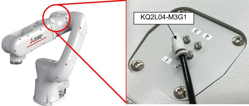
2) Connect the One-touch fitting and magnet gripper with a coil tube (TCU0425B-1).
