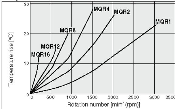
Note: Value when no pressure applied. Temperature rise is reduced by supply of air.
