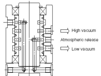
Using atmospheric release port
