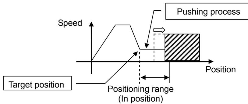
2) Movement of the workpiece in the direction opposite to the pushing direction
