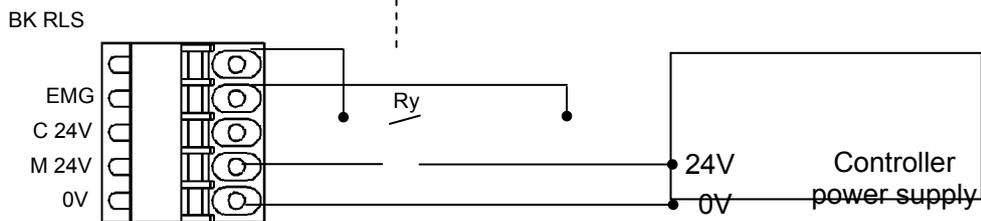
Power supply plug (the 3<sup>rd</sup> controller)
