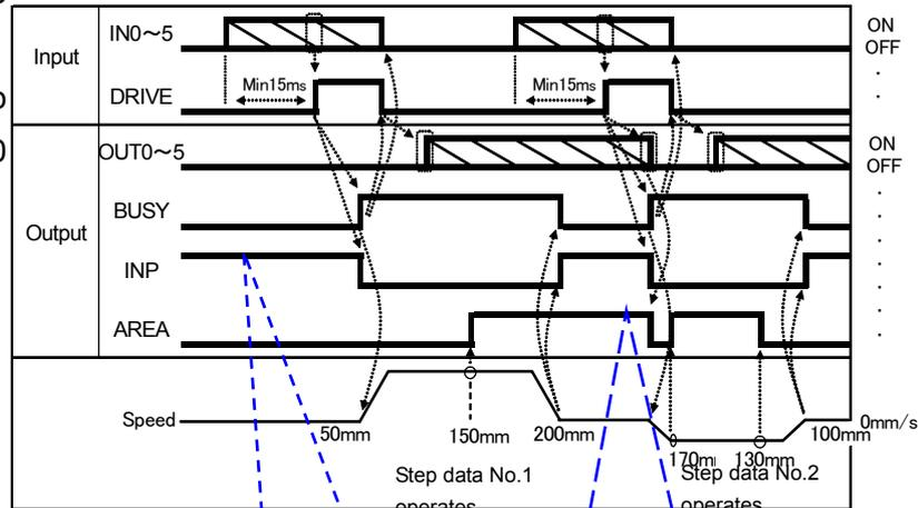
If the now position is inside of step data positioning, the INP signal is ON. Otherwise, the signal is OFF.
