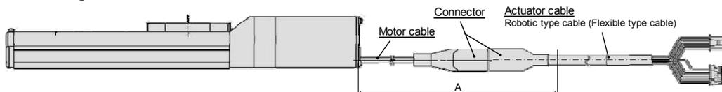
9. **Select “Robotic type cables” if the actuator cable will be repeatedly bent during operation. Do not put cables into a flexible cable duct with a radius smaller than the specified value. (Min. 50mm).**
