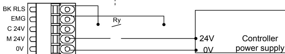
The relay must be a safety relay or monitored by a safety relay.
