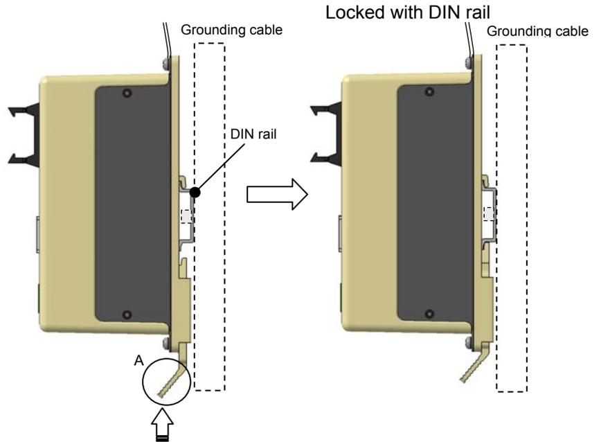
Hook the controller on the DIN rail and press lever A in the direction of the arrow to lock it.
