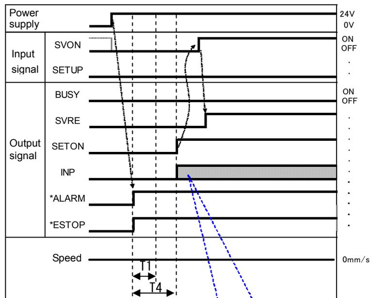
INP signal is ON when the current position is within the step data position range. If not, OFF
