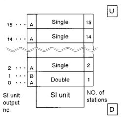
Fix the internal manifold wiring according to the type of solenoid valves to be mounted: single or double. Note that a single solenoid valve, in this case, cannot be output for a lack of internal wiring to solenoid B even if changed to double. The maximum number of the stations is 8 for 8 points of SI unit outputs, and 16 for 16 outputs provided that all the solenoid valves are single.
