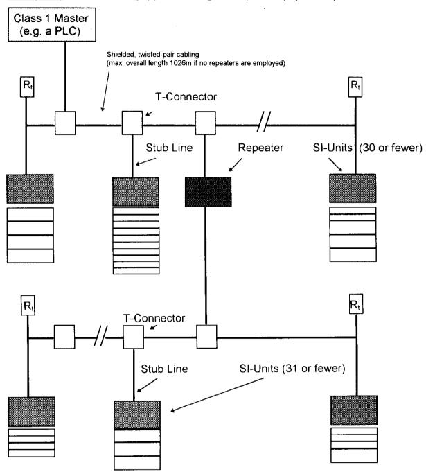
Note: A Class 1 master may also be inserted into the secondary PROFIBUS-DP loop. Throughout this manual, "master" will i nvariably imply a Class 1 Master, unless otherwise stated.
