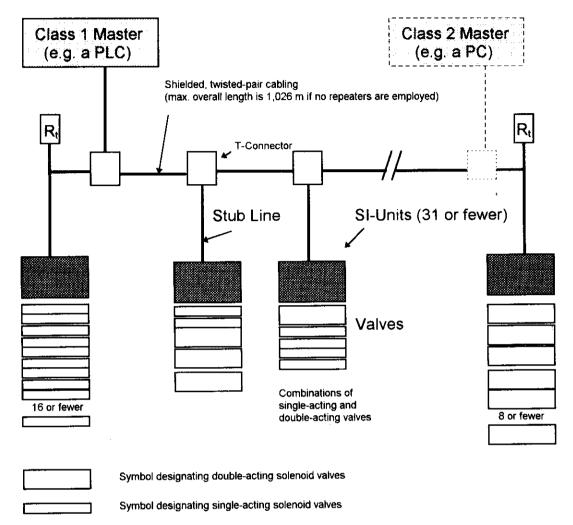
$R_{t}$ . Terminating resistors (120-150  $\Omega)$  required for RS-485 serial transmission
