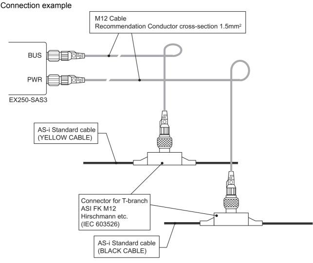
Neither M12 cable, As-i standard cable, nor connector for T-branch are supplied form SMC. Contact with each maker about the detail of the catalog etc.
