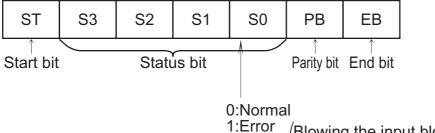
1:Error (Blowing the input block fuse or detecting) over current of input power supply
