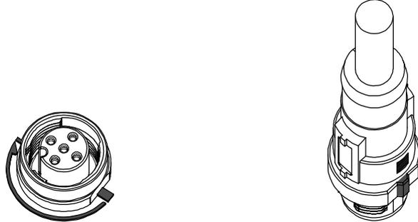
(2) Push the connector straight to insert it into the receptacle of the unit. If inserted without aligning the mark, the connector will not mate with the receptacle.
