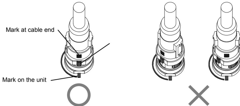
(3) Turn the connector clockwise. It stops when turned 1/4 turn. When the connector is turned 1/2 turn from the original position, the projected portion is set at the diagonal position to the mark and the turn is completed.
