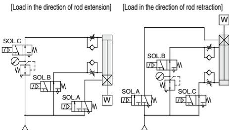
\* The symbol for the cylinder with lock in the pneumatic circuit uses SMC original symbol.
