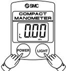
The auto power OFF function is canceled by activating the lock mode (auto power OFF cancel). When continuously pressed for 6 seconds or more, "L" is displayed on the LCD. Moreover, when the power is turned OFF, the lock mode is released.
