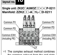
the common exhaust from the end plate and the direct exhaust from each station.
