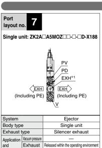
PD pressure has to be supplied with PV pressure.
