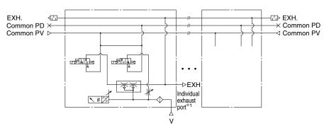
\*1 For the complex exhaust type, an individual exhaust port is provided to each station.
