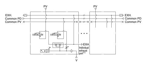
\*1 For the complex exhaust type, an individual exhaust port is provided to each station.
