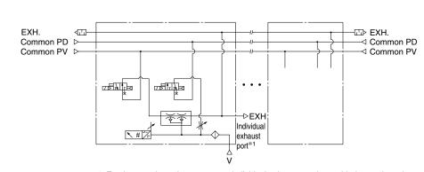
\*1 For the complex exhaust type, an individual exhaust port is provided to each station.
