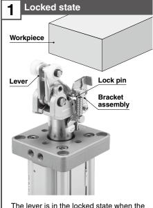
The lever is in the locked state when the lock pin is hooked on the bracket assembly.
