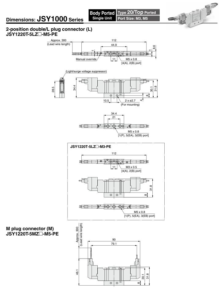
Non Plug-in Body Ported Single Unit (For Mounting P.E Plate)
