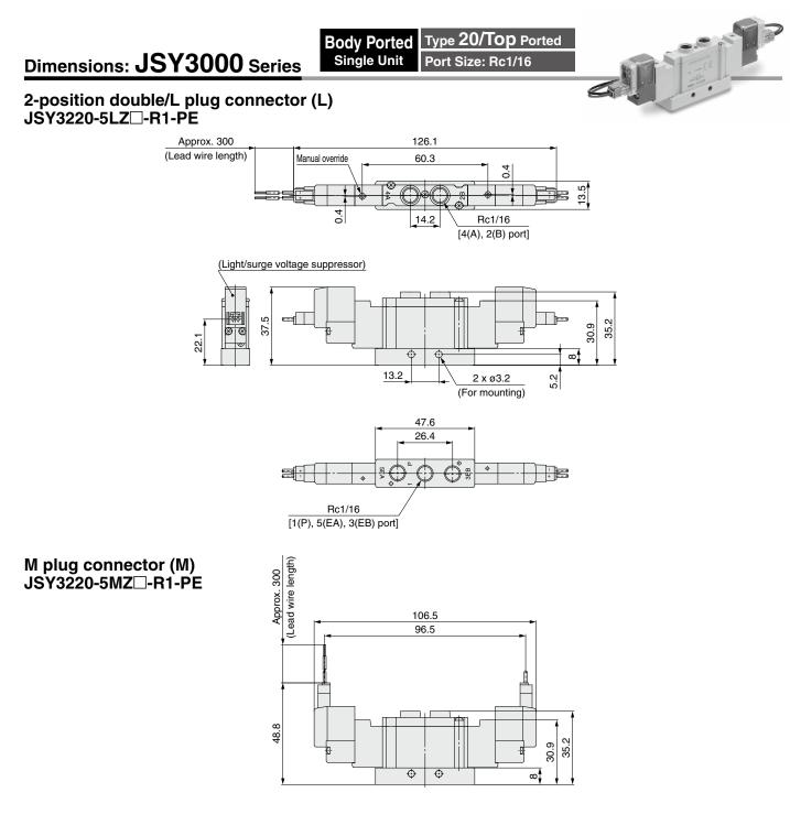
Non Plug-in Body Ported Single Unit (For Mounting P.E Plate)
