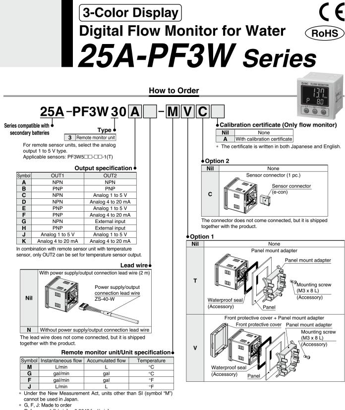
Reference: 1 [L/min]↔0.2642 [gal/min] 1 [gal/min]↔3.785 [L/min] °F = 9/5°C + 32
