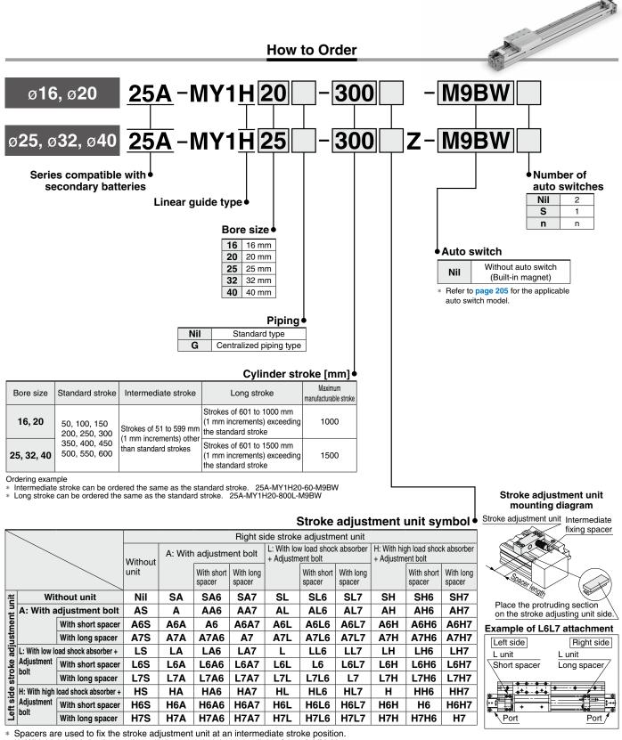
H: With high load shock absorber + Adjustment bolt is not available for 25A-MY1H16.
