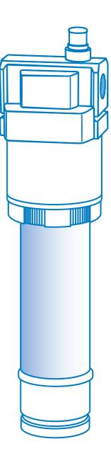
once again, membrane dried and then finally mist separated a third time. The air entering the system will have been dirty and humid, potentially containing tens-of-millions of particles of moisture, dust and other foreign contaminants.
