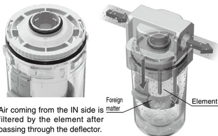
Air coming from the IN side is filtered by the element after passing through the deflector.
