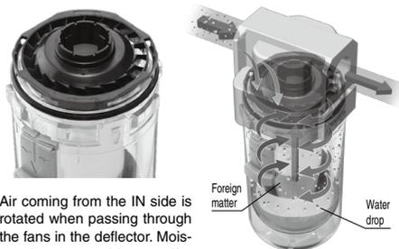
Air coming from the IN side is rotated when passing through the fans in the deflector. Moisture is separated by centrifugal force.
