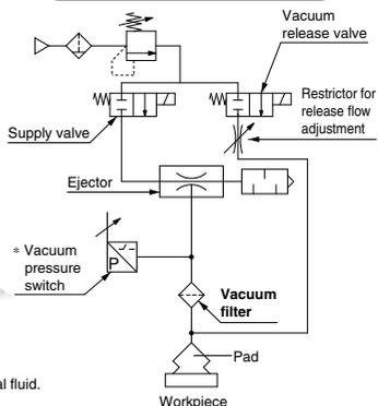
\* If water droplets enter to the vacuum pressure switch, use a vacuum pressure switch for general fluid. For handling, refer to Common Precautions and the Operation Manual.
