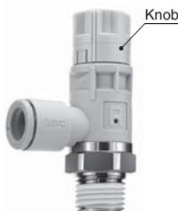
2. When performing the piping work, turn the tightening tool in the horizontal direction to the hexagon across flats of the body B so that any moment is not applied to the body A. If the tool is in contact with the body A, this may cause the body B to come off.
