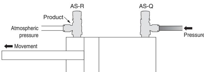
\* Adjust the product when the cylinder operates in the direction of the arrow or completes the operation.
