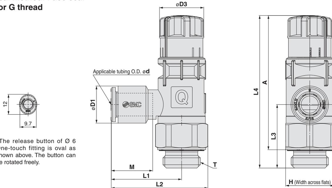
\* The release button of  $\varnothing 6$  One-touch fitting is oval as shown above. The button can be rotated freely.
