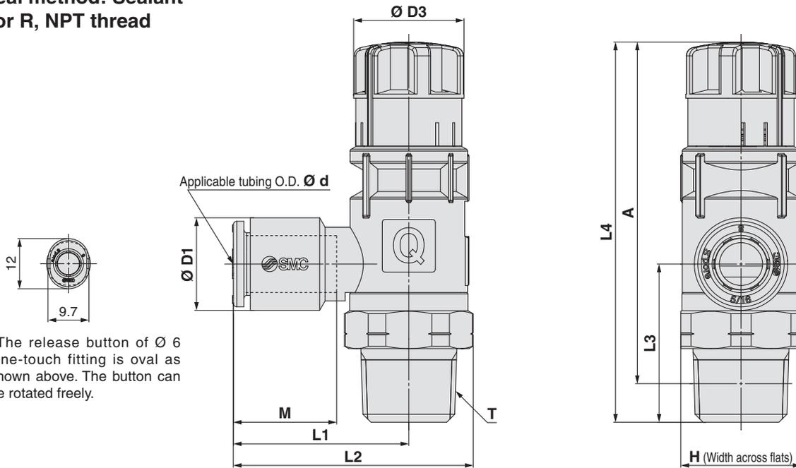
\* The release button of Ø 6 One-touch fitting is oval as shown above. The button can be rotated freely.
