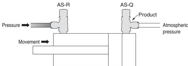
When the product mounted on the rod side is adjusted:
