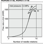
Note) The numbers above the flow rate characteristic curves in the charts show the applicable tubing outside diameter as defined by the product number.
