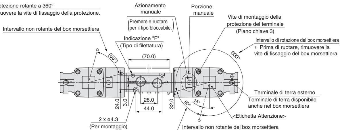
**Conformità ATEX****Elettrovalvola servopilotata a 3 vie**
