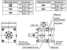
3. When installing the cylinder to machinery, etc., secure enough clearance and consider the mounting direction for manual lock release (releasing with the manual release bolt).
