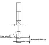
In order to further improve stopping accuracy, the time from the stop signal to the operation of the lock should be shortened as much as possible.
