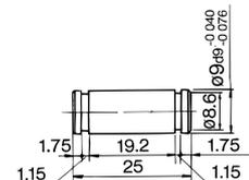
Retaining ring: Type C9 for axis
