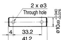
Retaining ring: Type C9 for axis
