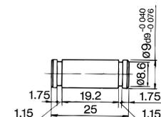
Retaining ring: Type C9 for axis
