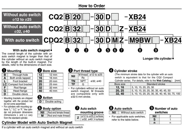
If a cylinder with an auto switch magnet and without an auto switch is required, there is no need to enter the symbol for the auto switch. (Example) CDQ2L32-25DZ-XB24
