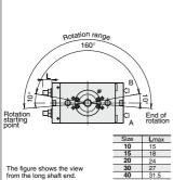
The rotation angle can be adjusted between 90° and 190°.
