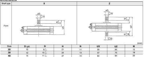
Note) Dimension parts different from the standard conform to the general tolerance.
