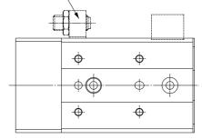
In case of without extension end adjuster type, port is plugged with a hexagon socket head screw at the time of shipment.
