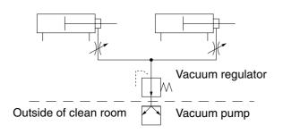
With an ejector When a few air cylinders are locally used.
