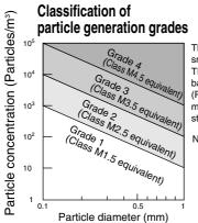
The grade classification is the SMC original method. The smaller the grade number, the less the particle generation. The upper concentration limit of the cleanliness class based on Fed. Std. 209E-1992 is shown in parentheses. (Refer to Front matter 23 "Particle generation measuring method" and Front matter 24 "Comparison of cleanliness standards" for details.)
