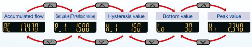
\* Either "Input of line name" or "Display OFF" can be added via the function settings.
