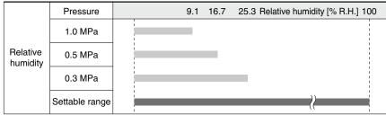
The range of atmospheric pressure and relative humidity that the switch can measure changes depending on the pressure inside the piping (under pressure). For example, if the pressure inside the pipe (under pressure) is 1.0 MPa and the relative humidity is 100% (maximum value), the atmospheric pressure relative humidity when released into the atmosphere will be 25.3%.
