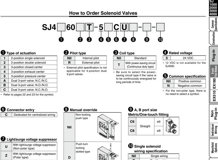
When the type with power-saving circuit is used, the non-polar type cannot be selected.
