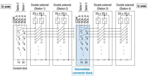
\* The U side solenoid valve with an intermediate connector block can be controlled.
