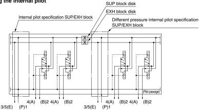
2. Different-pressure specification using the external pilot (For using the SUP/EXH block for external pilot)
