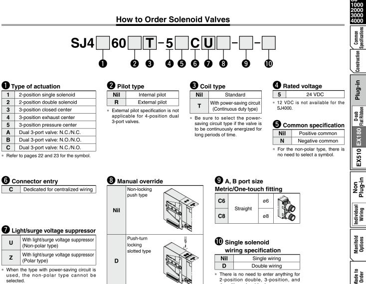
When the type with power-saving circuit is used, the non-polar type cannot be selected.
