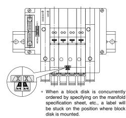
Different pressure internal pilot specification
