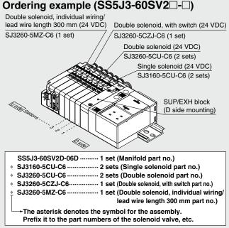
· For the valve arrangement, the valve closest to the D side is considered the 1st station. · Under the manifold part number, state the valves to be mounted in order starting with the 1st station as shown in the figure. If the arrangement becomes too complicated, specify the details on a manifold specification sheet.
