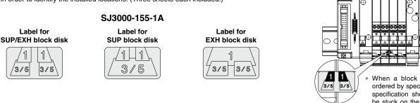
When a block disk is concurrently ordered by specifying on the manifold specification sheet, etc., a label will be stuck on the position where block disk is mounted.
