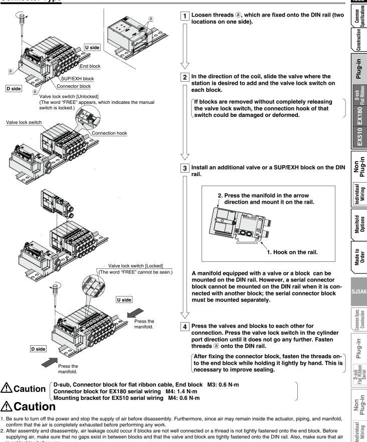
2. After assembly and disassembly, air leakage could occur if blocks are not well connected or a thread is not tightly fastened onto the end block. Before supplying air, make sure that no gaps exist in between blocks and that the valve and block are tightly fastened onto the DIN rail. Also, make sure that air is not leaking before use.
