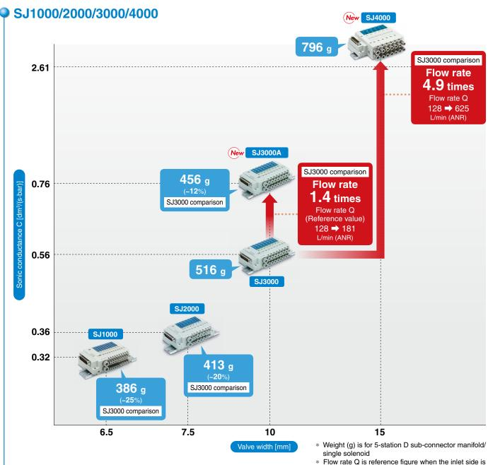
Flow rate Q is reference figure when the inlet side is 0.6 MPa, and the outlet side is 0.5 MPa (20°C)
