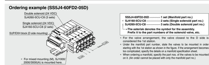
When SJ4000 and SJ1000/2000/3000 are mixed mounting (M), SJ1000/2000/3000 valves are mounted on the D side of SJ4000 D side SUP/EXH block.
