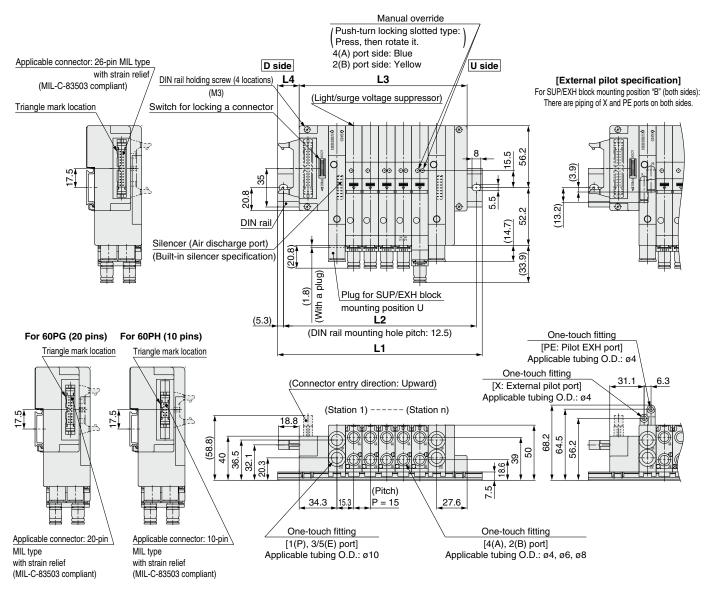
\* Type 60PG and 60PH differ only in their connectors, and the L1 through L4 dimensions are the same as type 60P.
