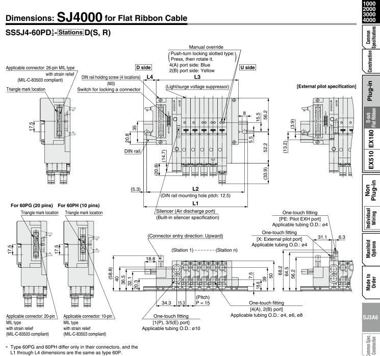
\* Type 60PG and 60PH differ only in their connectors, and the L1 through L4 dimensions are the same as type 60P.
