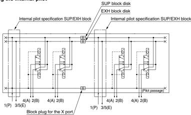
2. Different-pressure specification using the external pilot (For using the SUP/EXH block for external pilot)
