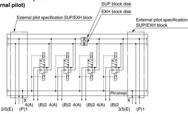
3. Different-pressure specification using the external pilot (For using the SUP/EXH block for different-pressure internal pilot specification)
