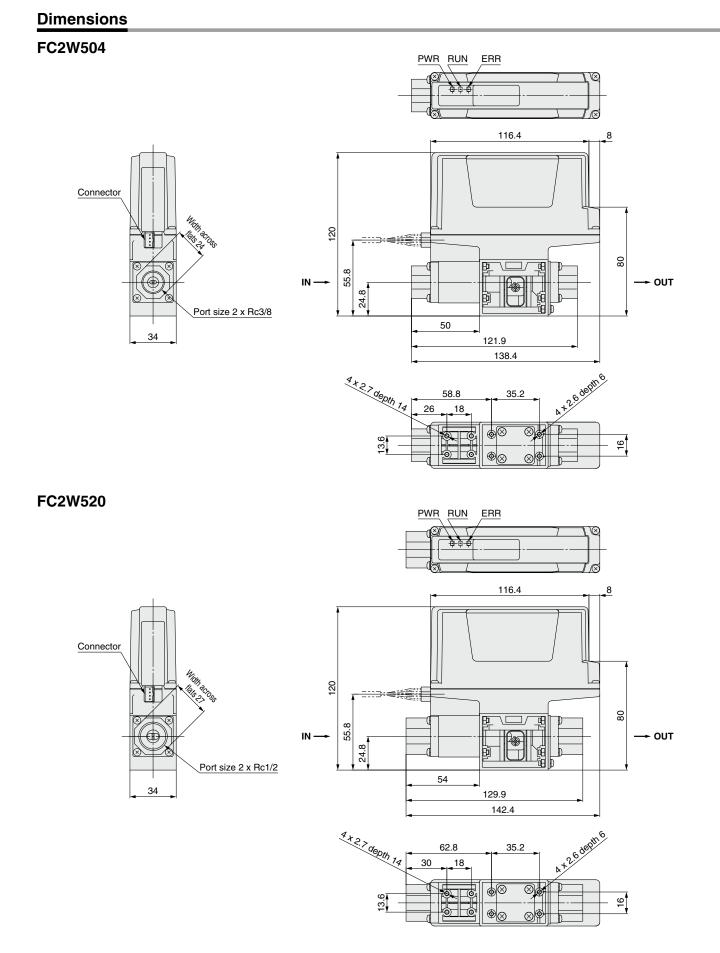
\* The piping on the IN side must have a straight section of piping whose length is 8 times the piping diameter or more.
