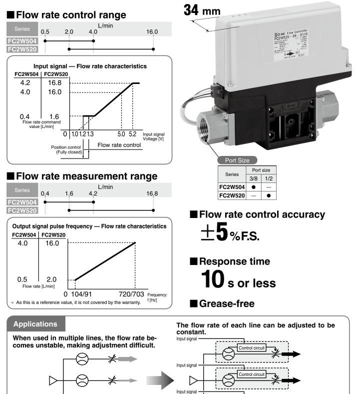
A single unit of the FC2W cannot provide complete shutoff. To stop the flow in an emergency, a 2 port valve is required. Refer to the next page for details.
