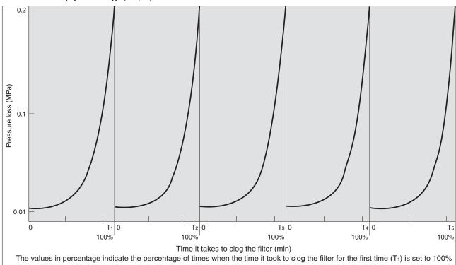
Introduce a certain concentration of dust and back-flush the filter when the pressure loss reaches 0.2 MPa. Repeat filtering and back-flushing process (up to five times shown in the graphs).
