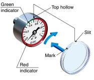
3. After completing the setting, replace the cover. Attach the cover by aligning the cutout in the cover to the groove on the top of the silver case. Turn the cover clockwise until it stops. Make sure that the matching
