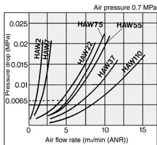
(Example) To get pressure drop at 0.3 MPa of air pressure, 5 m<sup>3</sup>/min (ANR) of air flow and model HAW75-20, use  $\Delta P = 0.0065$  MPa at 0.7 MPa from the table and convert P<sub>1</sub> to 0.3 MPa.
