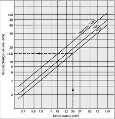
Note) If the hydraulic pump motor output is 30 kW and the heat loss is 55%, the required conversion volume is 16.5 kW. (Select the heat loss percentage based on the hydraulic circuit.)
