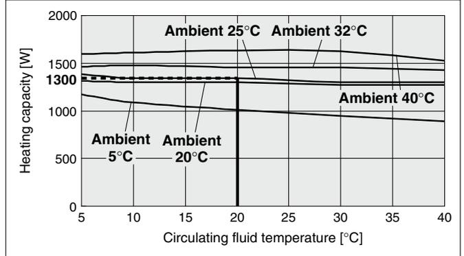
**HRS060-A-20 (Single-phase 200 to 230 VAC) (50 Hz)**
