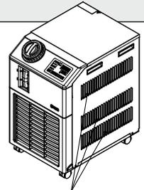
Ventilation slots are added to side panels (on both sides).
