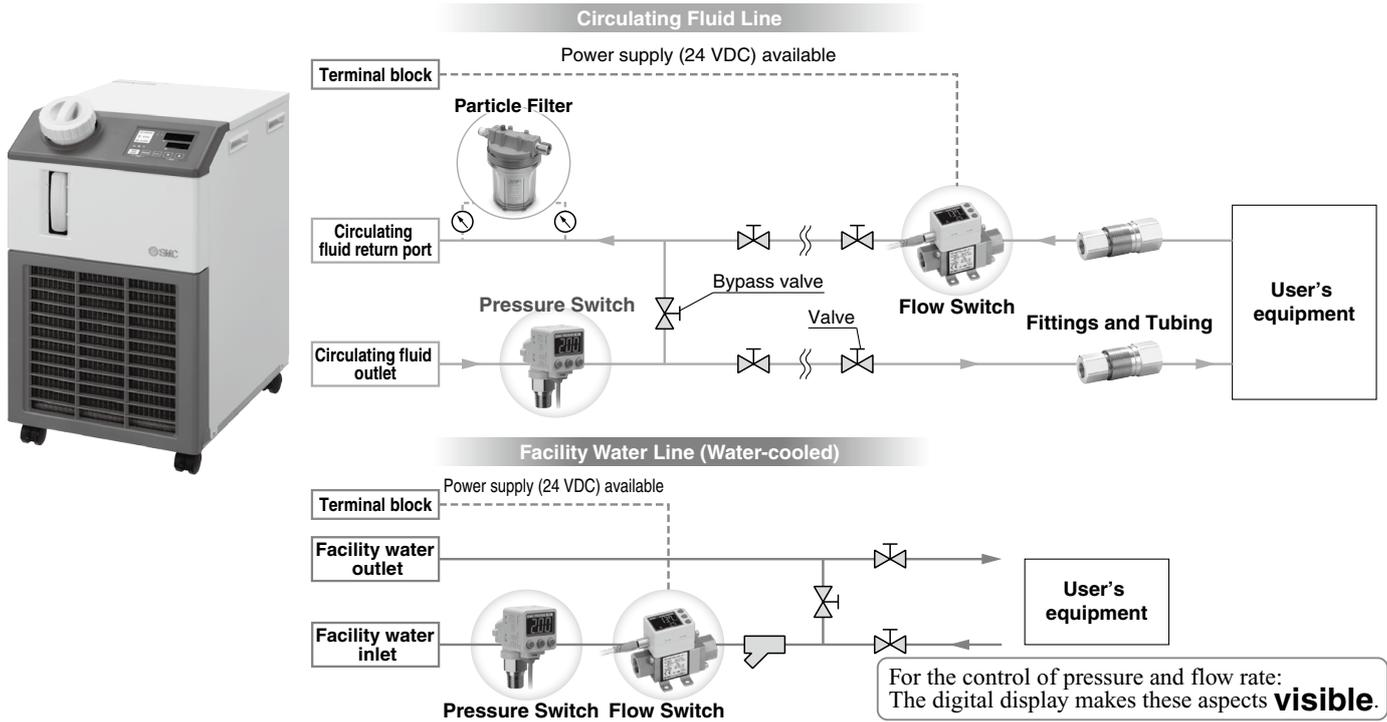
**Flow Switch:** Monitors the flow rate and temperature of the circulating fluid and facility water. Refer to the Web Catalog for details.
