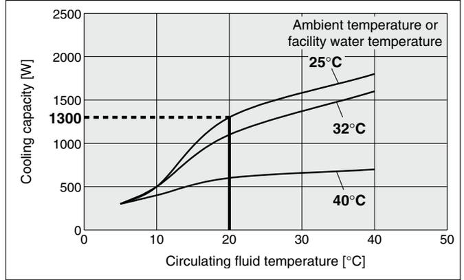
**HRS018-A-10, HRS018-W-10 (Single-phase 100/115 VAC) (50 Hz)**
