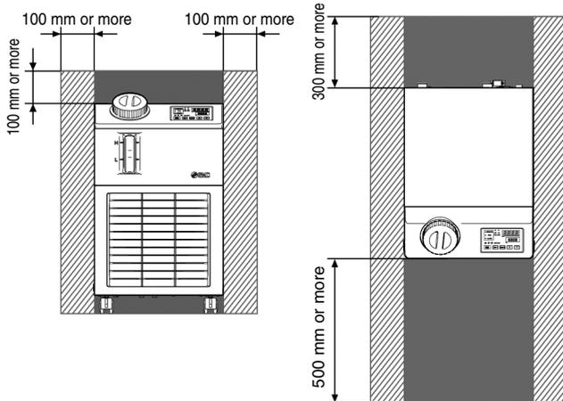
When option G, high-temperature environment specification, is selected: HRS030/HRS040/HRS050/HRS060 (A ventilation space is required since the ventilation slots are provided on the sides of the product.)
