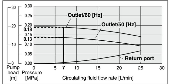
**HRS<sup>030</sup><sub>040</sub>-A<sub>W</sub>-20** (Single-phase 200 to 230 VAC)
