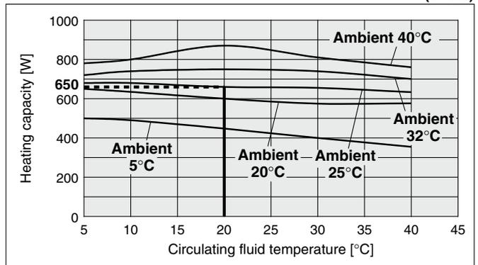
**HRS030-A-20** (Single-phase 200 to 230 VAC) (50 Hz)
