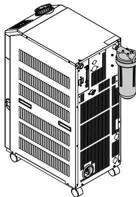
The following reference drawing shows the HRS-PF004 mounted on the HRS050/060. For details, refer to the dimensions or the Operation Manual.
