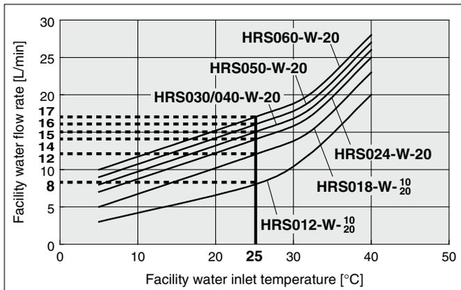
\* This is the facility water flow rate at the circulating fluid rated flow and the cooling capacity listed in the "Cooling Capacity" specifications.
