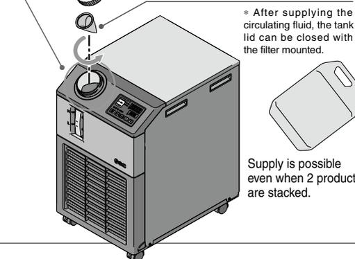
\* After supplying the circulating fluid, the tank lid can be closed with the filter mounted.
