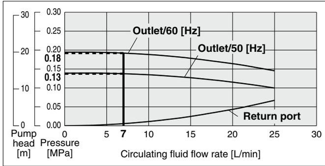
**HRS<sup>012</sup><sub>018</sub>-A<sub>W</sub>-20** (Single-phase 200 to 230 VAC)
