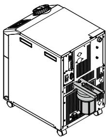
The following reference drawing shows the HRS-PF001 mounted on the HRS012 to 024. For details, refer to the dimensions or the Operation Manual.
