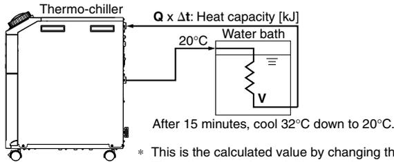
\* This is the calculated value by changing the fluid temperature only. Thus, it varies substantially depending on the water bath or piping shape.
