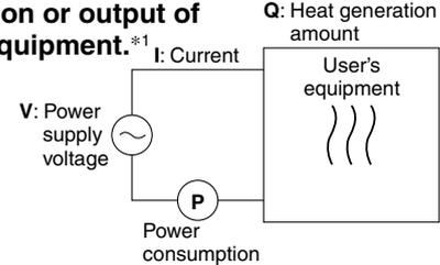
\*1 The examples above calculate the heat generation amount based on the power consumption. The actual heat generation amount may differ due to the structure of the user's equipment. Be sure to check it carefully.
