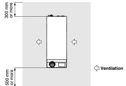
3. If it is impossible to exhaust heat from the installation area indoors, or when the installation area is conditioned, provide a duct for heat exhaustion to the air outlet port of this product for ventilation. Do not mount the inlet of the duct (flange) directly to the air vent of the product, and keep a space larger than the diameter of the duct. Additionally, consider the resistance of the duct when making the air vent port for the duct.
