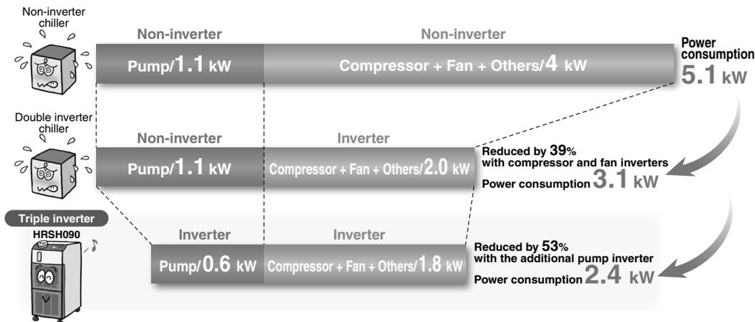
Operating ratio: Ratio of 9.5 kW (with heat load) to 0 kW (without heat load) Operating ratio: 50%, with heat load of 9.5 kW all the time
