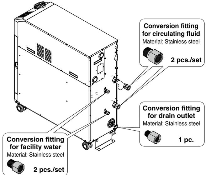
When option J (With automatic fluid fill function) is included, use the following part numbers.
