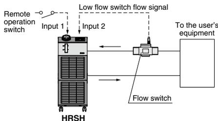
Power for flow switches (24 VDC) can be supplied by the thermo-chiller.
