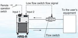
Power for flow switches (24 VDC) can be supplied by the thermo-chiller.
