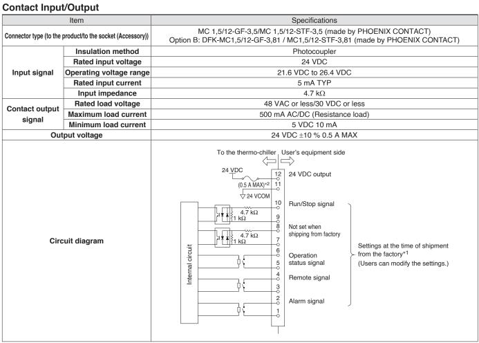
\*1 The pin numbers and output signals can be set by the user. For details, refer to the Operation Manual.
